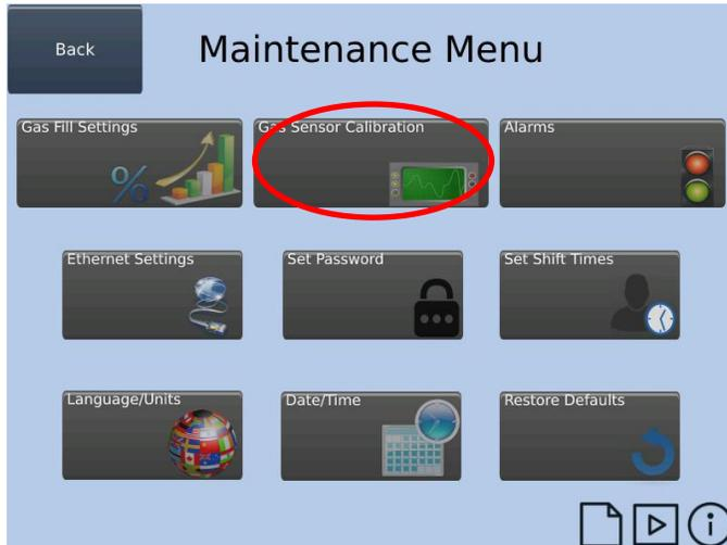
**Note:** *Gas sensor calibration is strongly recommended every 30 days. A daily reminder (calendar icon) will appear on the ‘Operator Screen’ if the calibration is past due. The reminder can be bypassed, one day at a time, for 30 days. But, the line will not operate if the calibration is 60+ days past due.*
