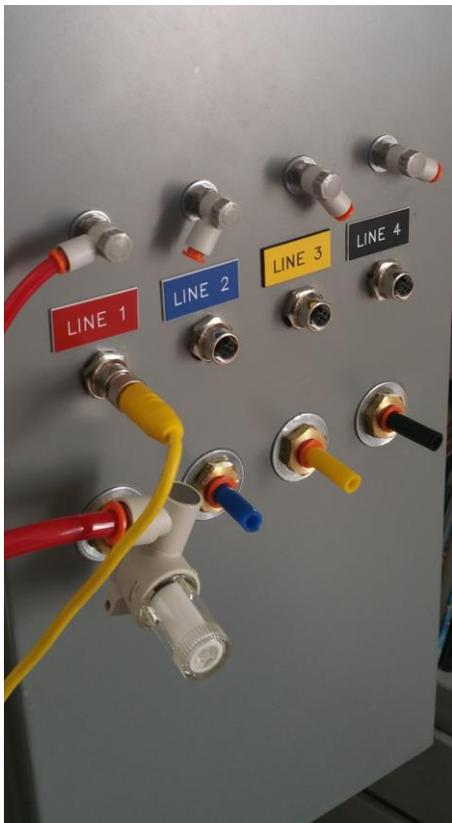
5. Connect each tubing set to the corresponding "Line #" color on the side of the AFS Machine. Ensure the filter is properly installed on the vacuum tubing (as shown). An arrow on the filter housing indicates direction of flow (toward the AFS machine).
